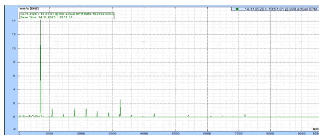
Fig.6-4. Spectra of the oscillations at several points of the frame, example-4.
