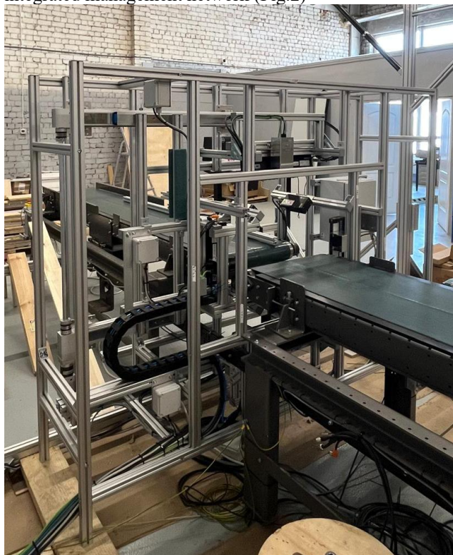
Fig. 2. Actual prototype of the scanner system with 4 triangulation and 4 visual cameras and a translation system for optical alignment (Source: authors created based on SIA LV Timber data)
