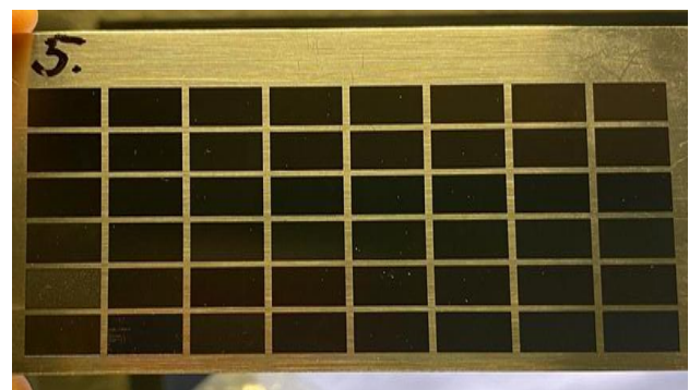
Fig. 5. Plate with matrix from the tests of the quality of roughness of the marking
