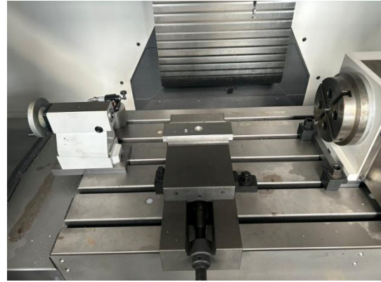
Fig. 3. Table, vise and 4 th axis
