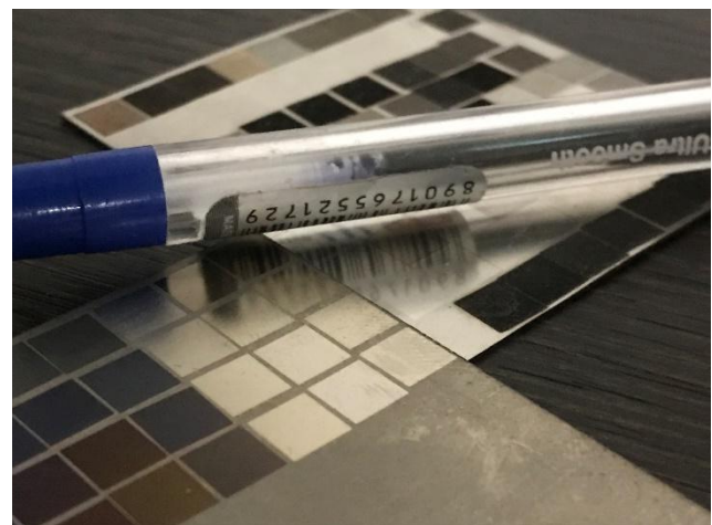
Fig. 1. Laser polished surface reflection of titanium alloy (left-bottom) and AISI 316L stainless steel (top right) samples
