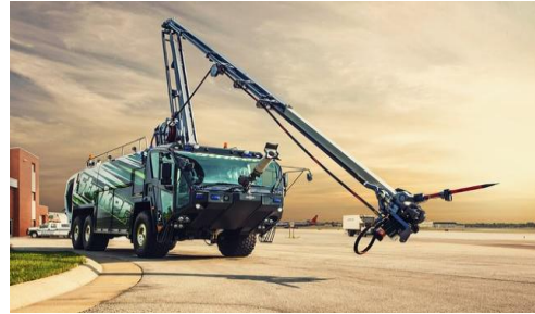
Fig. 2. Firetruck with Oshkosh robotic arm with Snuzzle
