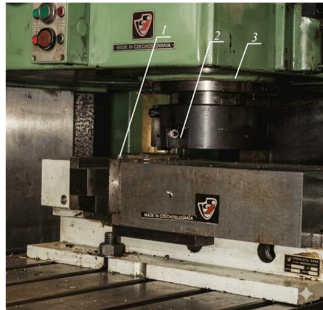
Fig.1 Experimental setup. 1-workpiece, 2- tool, 3-machine TOS FD 40
