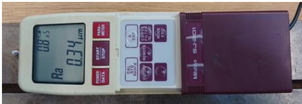
Fig.3 General view of the roughness meter Mitutoyo SJ201 P/M
