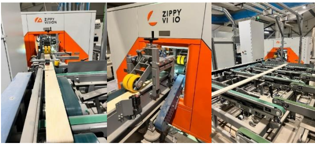
Fig. 2. Board fixing and feeding mechanism (Source: authors created based on SIA LV Timber data).
